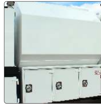
New 8D flat-sided oval diesel tank saves weight - the cabinets under 8D tank are all-aluminum
