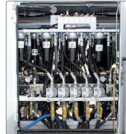
New design improves serviceability on the high pressure filters
