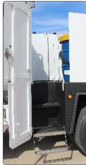
New center deck access - wider with illuminated stairway & 3-point contact
