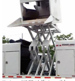
Massive quad (4) "X" style lift scissors with four corner lift provide exceptional hopper stability especially when dumping wet, unbalanced or sticky debris.
