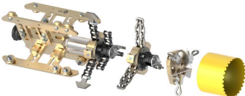
**Kettenschleuder 1/4" - 1" | Chain scrapers 1/4" - 1" | Têtes à chaînes 1/4" - 1"**
