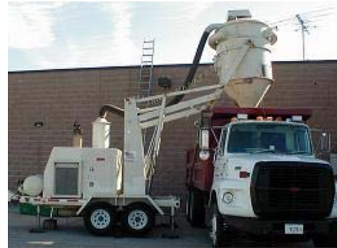
Mini-VecLoader Loading into a Dump Truck
